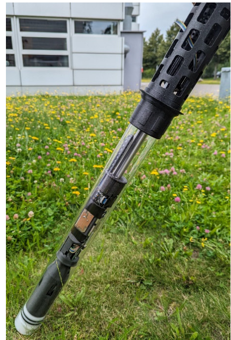
Figure 7: Minirhizotron with integrated automated mechanics, without weatherproof head cover.
