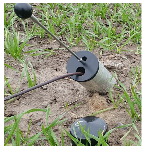
Figure 3: Tube installed at a 45° angle, darkened above ground, with CI600 inserted
