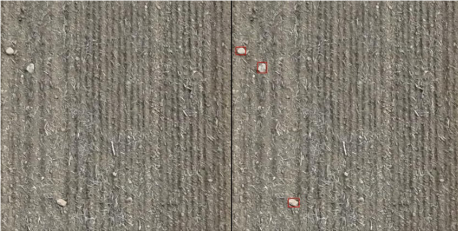
Figure 2: Raw image slice (left) and bounding boxes of detected stones (right)
